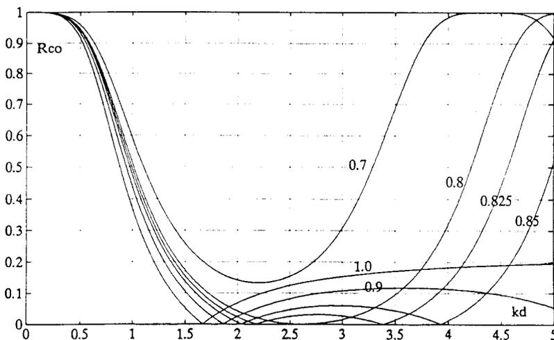
Co-polarized reflection coefficient for a plane wave incident to a layer of bi-isotropic medium with a conductor backing, as a function of normalized thickness  $kd$ . The normalized impedance has the value  $\eta/\eta_o = 0.8$  and the normalized Tellegen parameter varies between  $\chi_r = 0.7 \dots 1.0$ . It is seen that the co-polarized reflection is small for a wide band when  $\chi_r$  has a value slightly larger than  $\eta/\eta_o$ .
